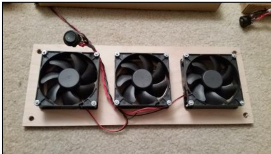
Back of system, showing fan assemblies
